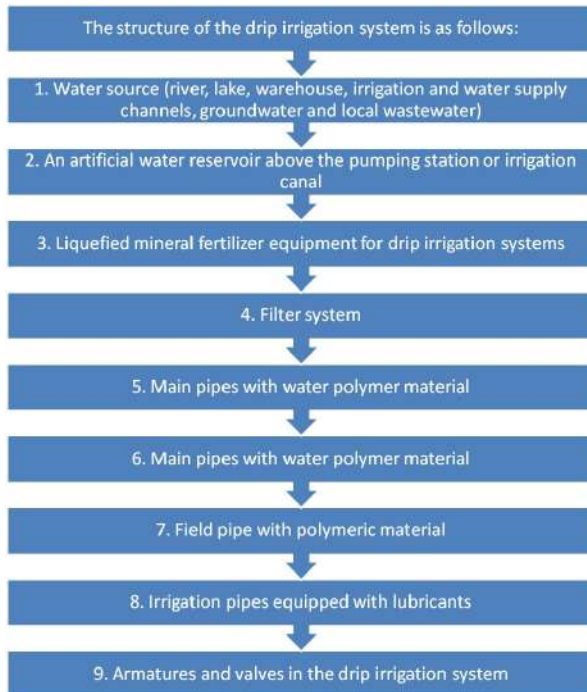
Figure 1. Structure of the drip irrigation system
